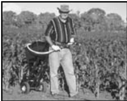
Peter Gregg using a battery powered sprayer designed for application of Helicoverpa attractant formulations
