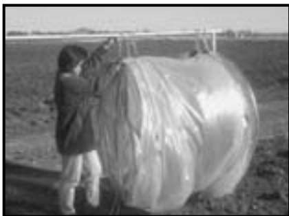
Alice Del Socorro setting up a field wind tunnel for experiments on Helicoverpa attractants.
