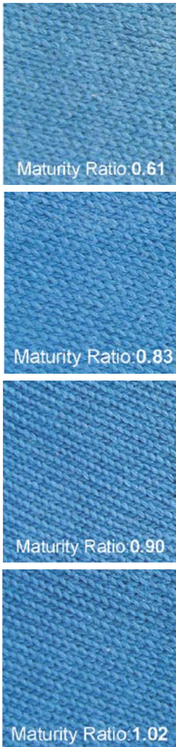
Figure 10.2: Immature cotton fibres with low Micronaire (associated with maturity ratios less than 0.85) and will dye a lighter hue and will abrade more readily and give a poorer appearance. Micronaire is generally associated with immature fibre (see chapter 3 on fibre biology for definitions). (Photos: CSIRO).
