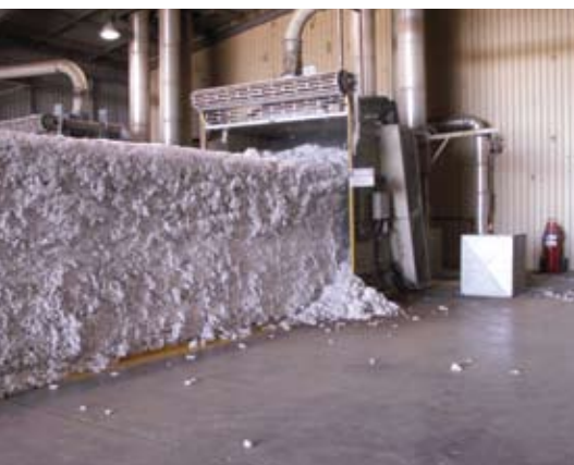
Figure 13.2: The module bay is an important intervention point for removing non-cotton contamination from modules. (Photo: CSIRO).
