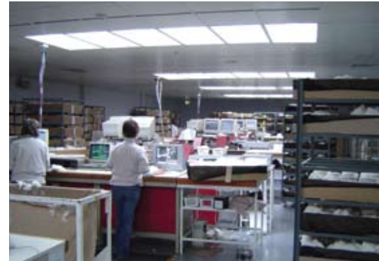
Figure 13.8: Modern classing rooms use both traditional classing methods and HVI to grade cotton and establish fibre quality traits essentially for marketing and for spinning mill requirements. (Photo: CSIRO).
