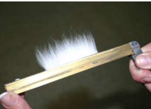
Figure 6.2: Photo of a fibre array comb for the HVI Fibrograph (length) and strength tester. (Photo: Warwick Stiller, CSIRO).
