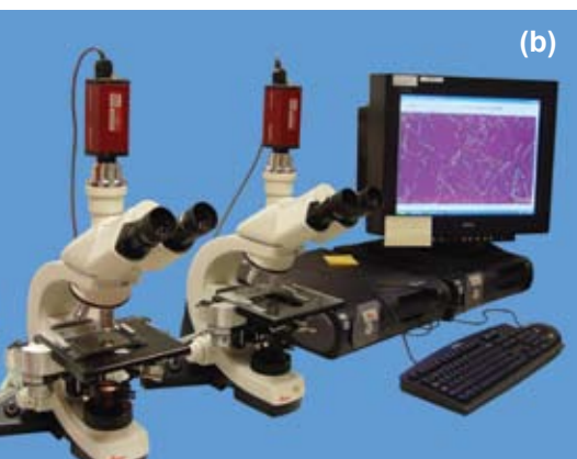
Figure 6.8: New instrumentation has been developed that offers significant opportunities to measure fibre linear density (a - Cottonscan™) and fibre maturity ratio (b - SiroMat) directly and quickly as an alternative to the indirect measurement of these properties using Micronaire. (Photos: CSIRO).
