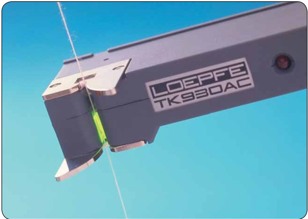
Figure 7 – Yarn clearer to remove foreign matter from yarn in winding and open end spinning (photo courtesy of CSIRO Materials Science and Engineering)
