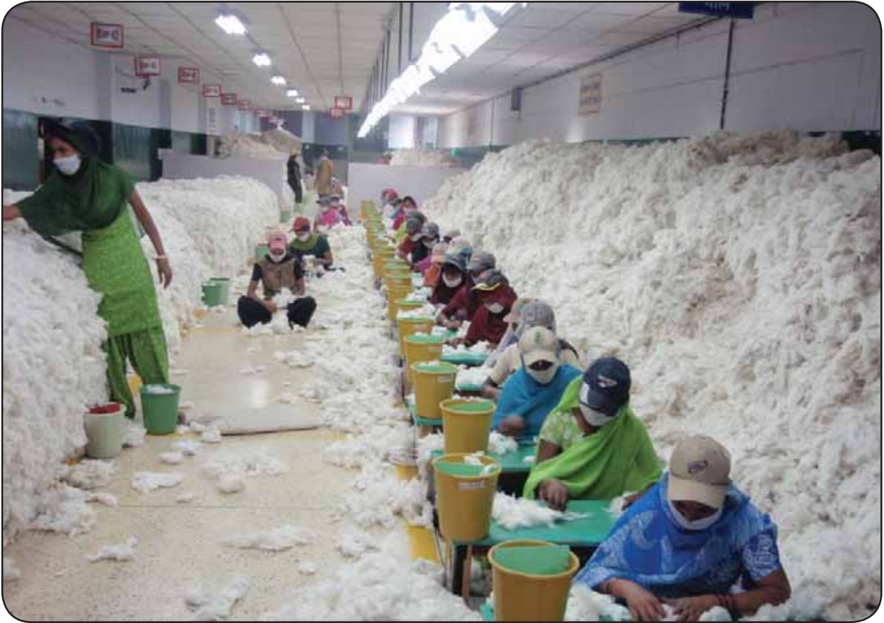
Figure 5 – Manual removal of contaminants from cotton before release to spinning mill (India)
