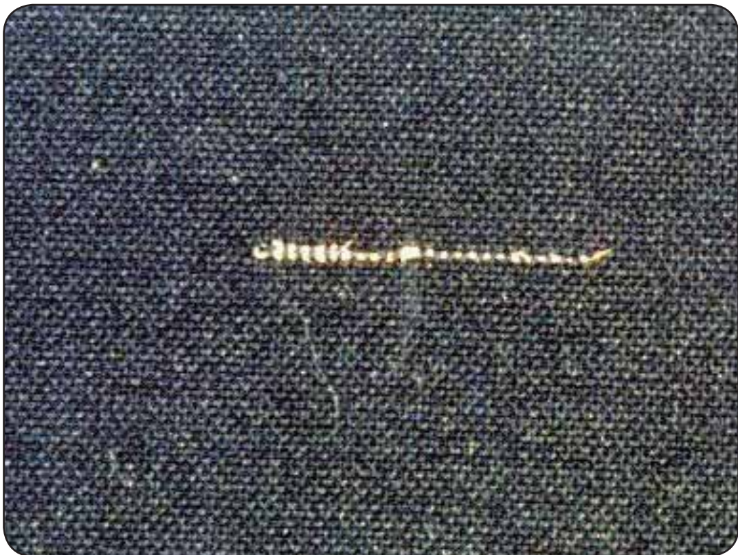
Figure 2 – Contaminated Fabric (photo courtesy of CSIRO Materials Science and Engineering)
