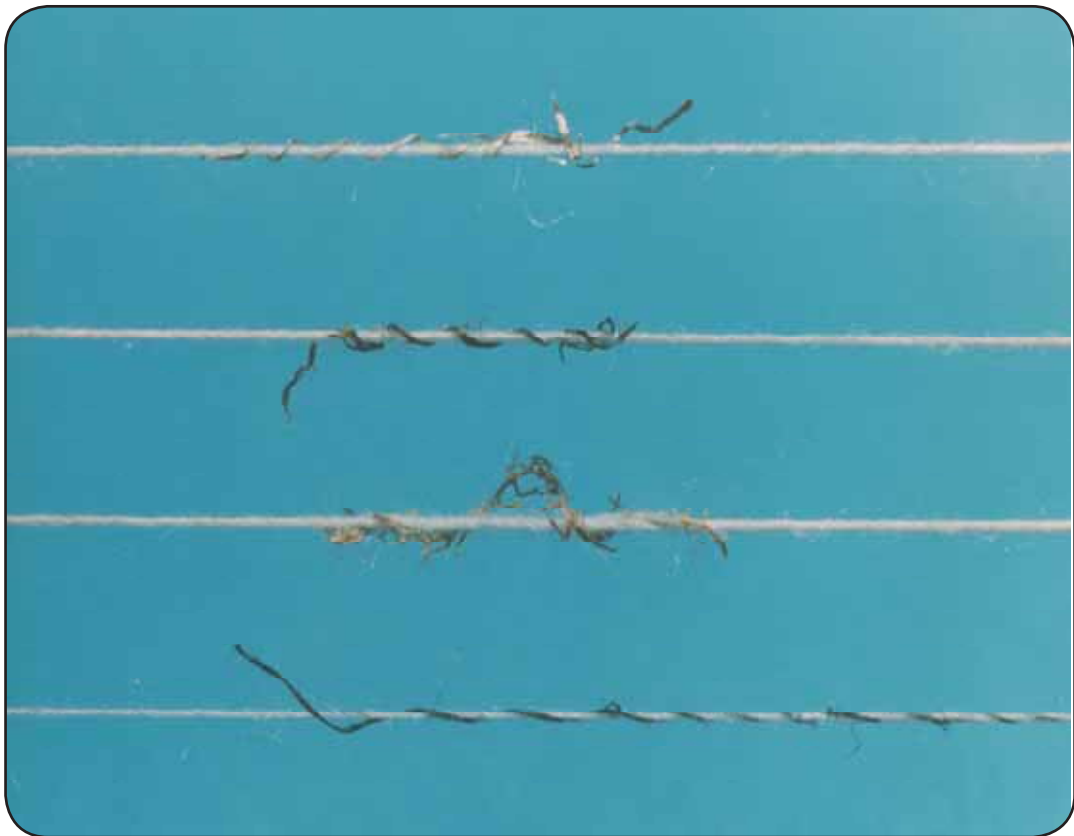
Figure 1 – Contaminated Yarns (photo courtesy of CSIRO Materials Science and Engineering)
