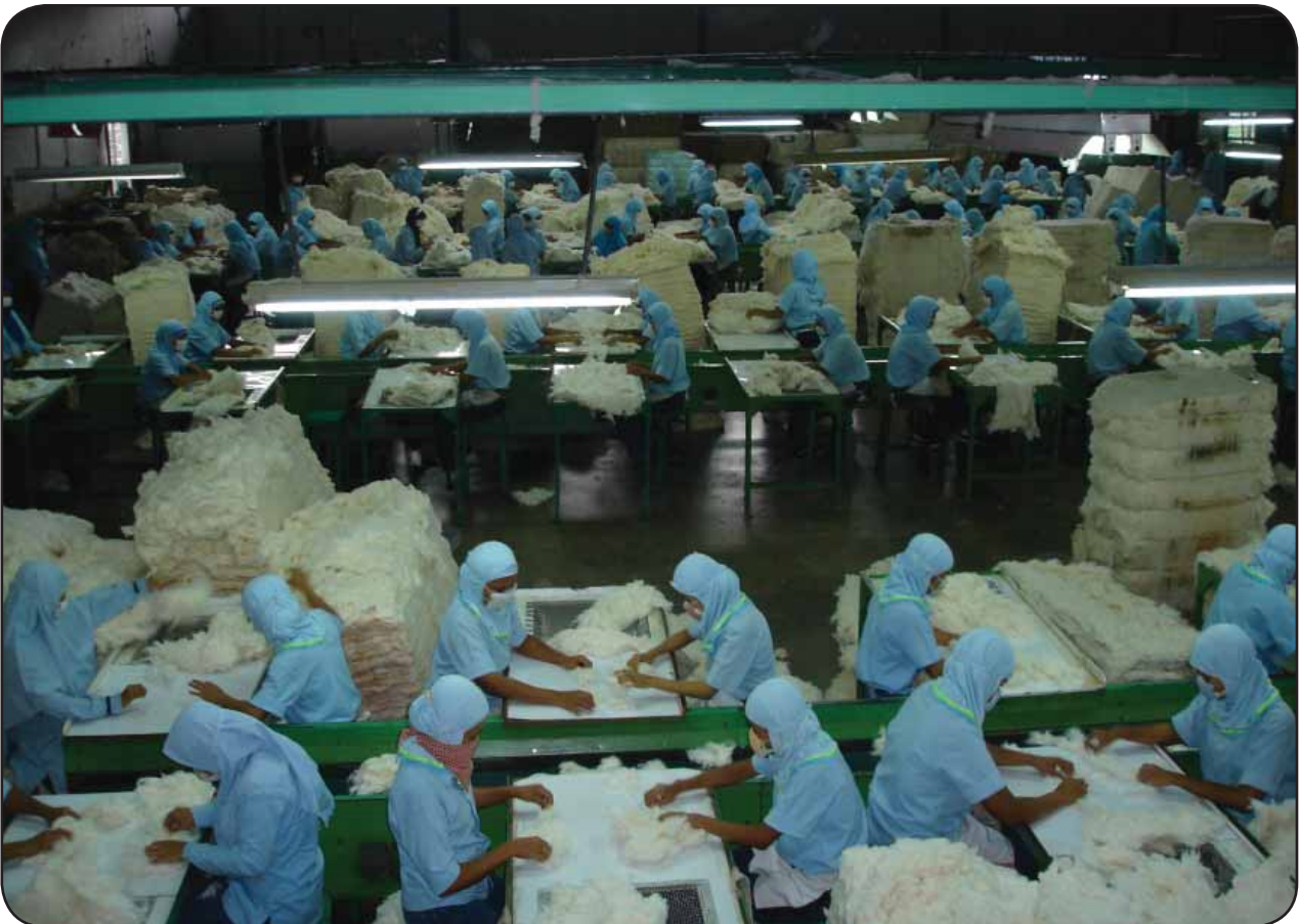
Figure 4 – Manual removal of contaminants from cotton before release to spinning mill (Indonesia)
