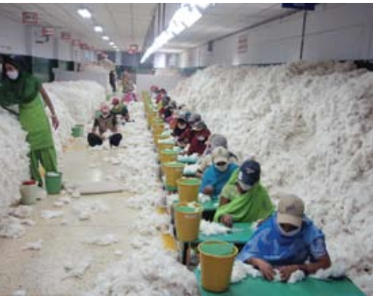
Figure 1.2: Some spinning mills invest significantly to remove contamination. This shows manual decontaminating cotton before processing at an Indian Spinning Mill. (Photo: Rene Van der Sluijs, CSIRO).
