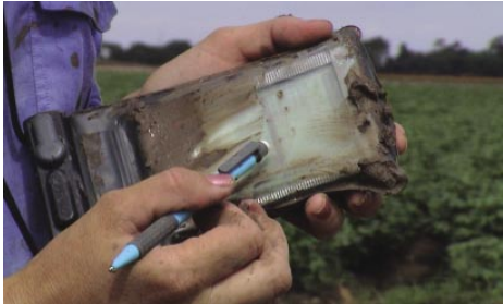
A waterproof pouch can be used to protect the handheld device.
