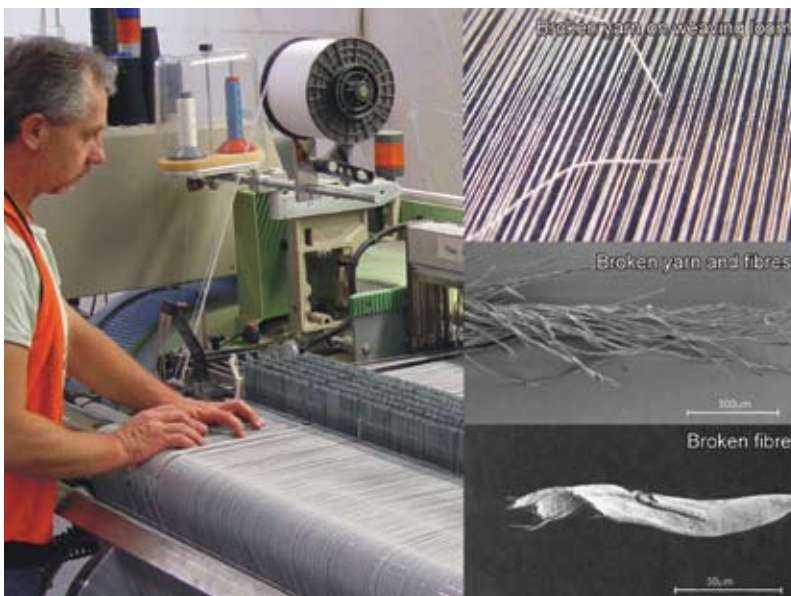
Figure 8.1: Strong fibres resulting from appropriate variety selection and by avoiding situations which delay crop maturity (which may result in more immature fibre that weakens the fibre) will avoid broken fibres which lower yarn and fabric quality. (Photos: CSIRO).
