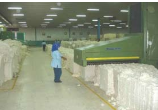
Figure 5.4: A 'laydown' takes the cotton from opened bales of differing quality. (Photo: Rene Van der Sluijs, CSIRO).
