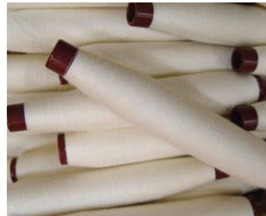
Figure 5.8: Ring Spinning produces the yarn which is wound onto bobbins. (Photos: CSIRO).
