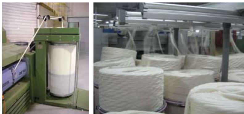
Figure 5.5: Carding produces a sliver a single continuous strand of overlapping fibres. (Photos: CSIRO).
