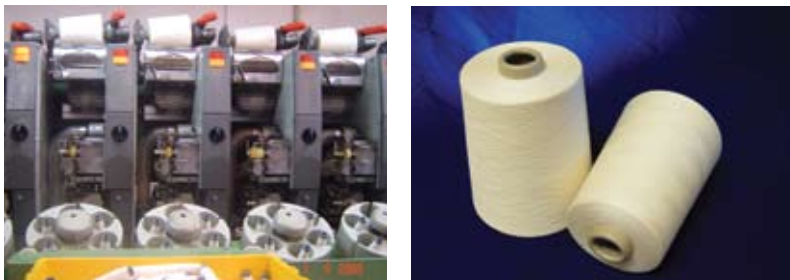
Figure 5.9: Winding produces a yarn package. (Photos: CSIRO)
