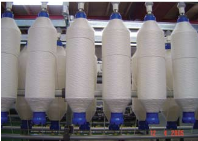
Figure 5.7: Roving bobbins on the creel of a ring spinning machine. The formation of roving reduces the sliver into a finer strand with the addition of twist. (Photo: CSIRO).
