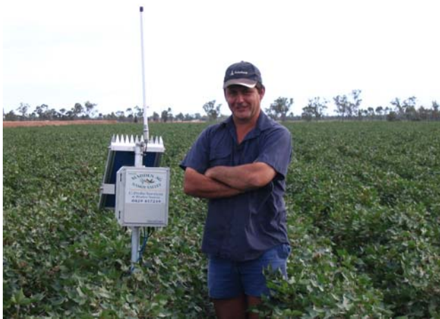
Above: Cotton Grower Paul Hawkins measuring soil moisture with a capacitance probe
