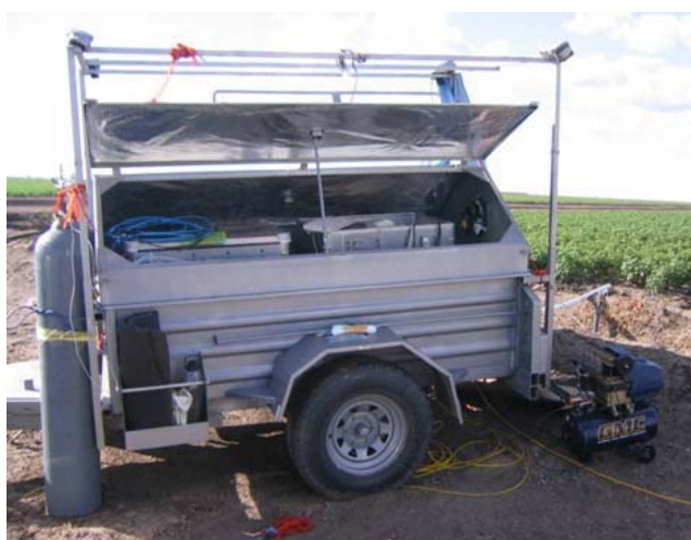
Above: Monitoring equipment used to track the greenhouse gases from a cotton crop on the farm trial.
